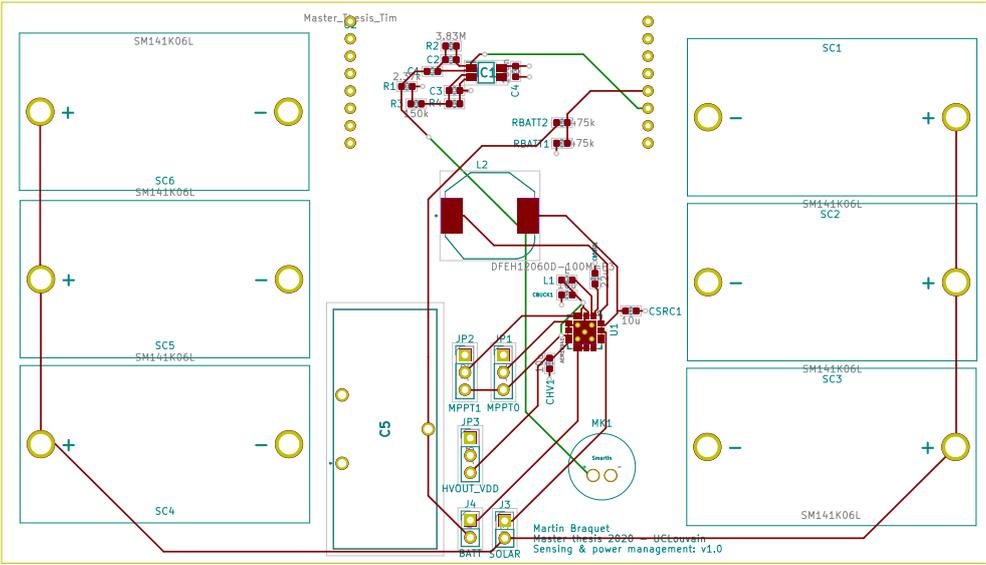
Figure C.1: PCB layout
