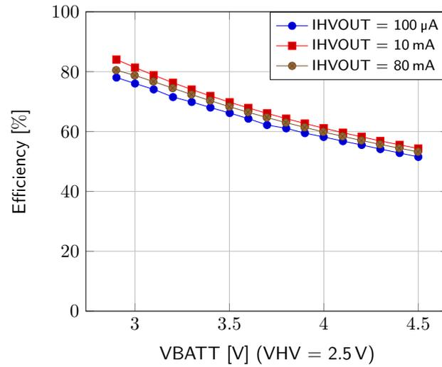
Figure 4.4: High-voltage LDO efficiency at 2.5 V in function of the load current
