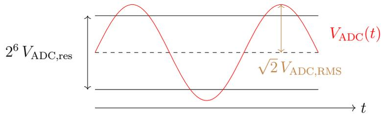
Figure 5.6: Resolution and RMS values of ADC voltage
