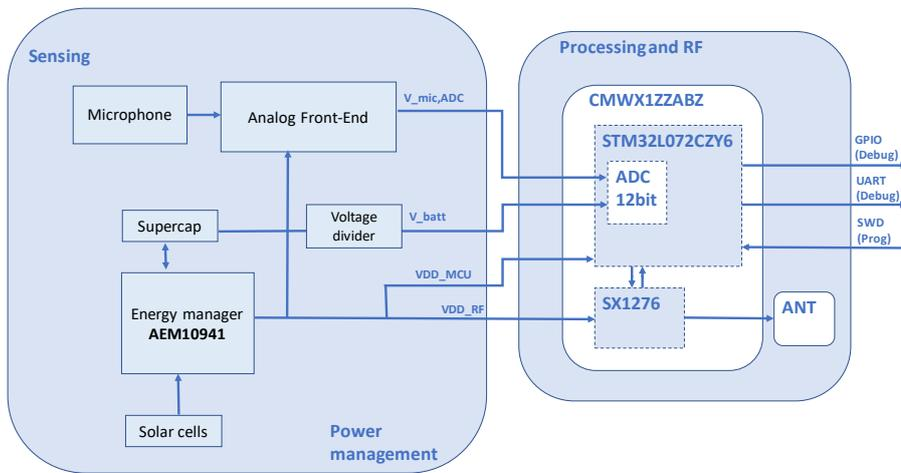
Figure 8.1: Electronics diagram of the final model
