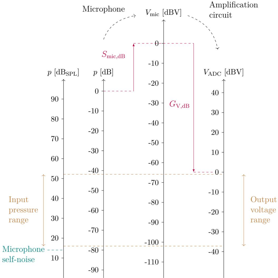
Figure 5.7: Range of  $p$ ,  $V_{mic}$  and  $V_{ADC}$  along the dB scale
