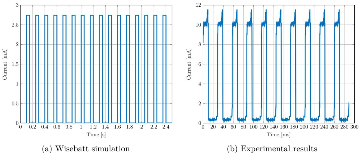
Figure 7.1: Current consumption of the CMWX1ZZABZ without TX/RX
