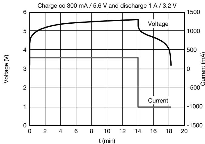
Figure 7.11: Constant current charge and discharge: 90 F / 5.6 V [23]
