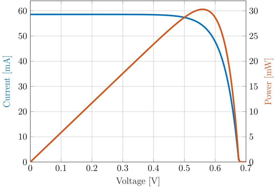
Figure 7.4: IV and PV curves of a typical solar cell: SM141K06L
