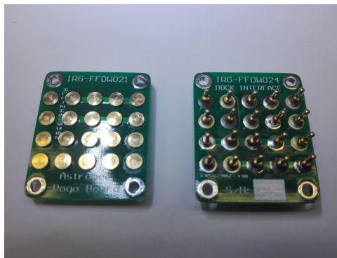
Figure 5: Soldering of the Astrobee Pogo board and Dock Pogo board
